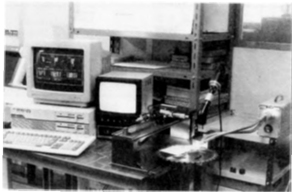
Fig.2 View of the tooth shape measurement apparatus.
