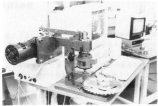
Fig.1 Peeling test apparatus.
